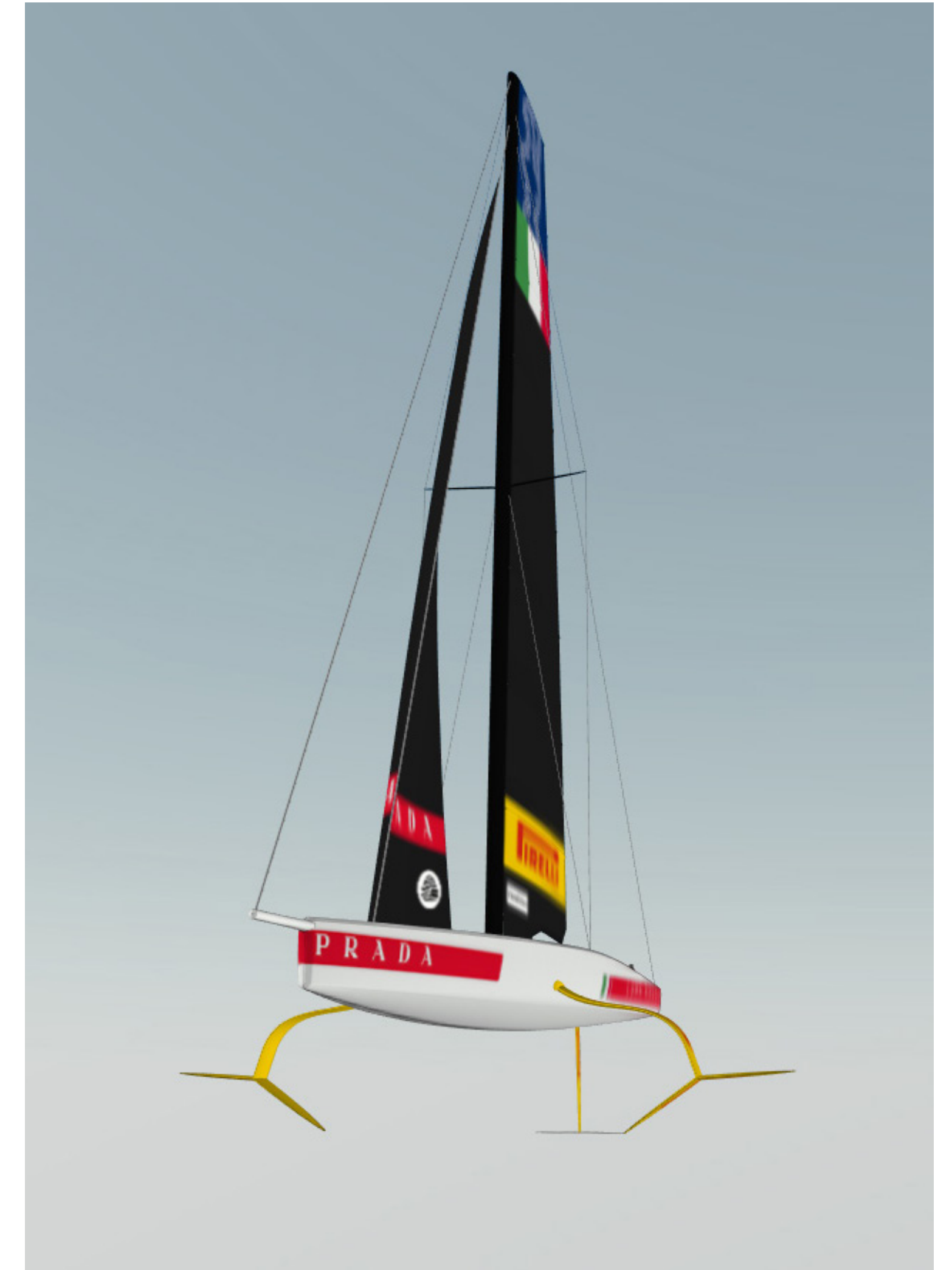
Maximum stability: foils lowered during manoeuvring
