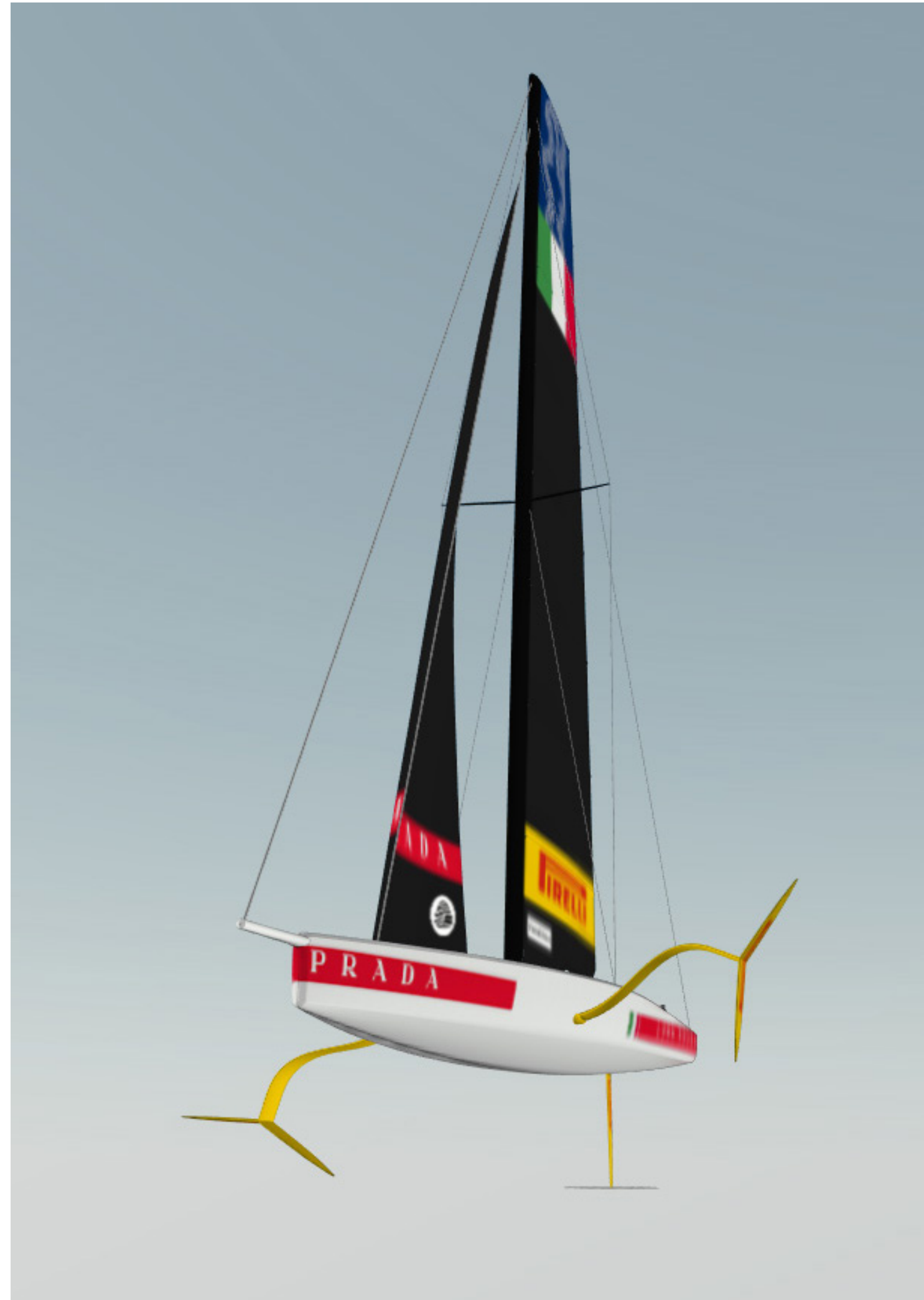
Foiling mode: the leeward foil raises the hull, the windward foil provides positive righting moment
