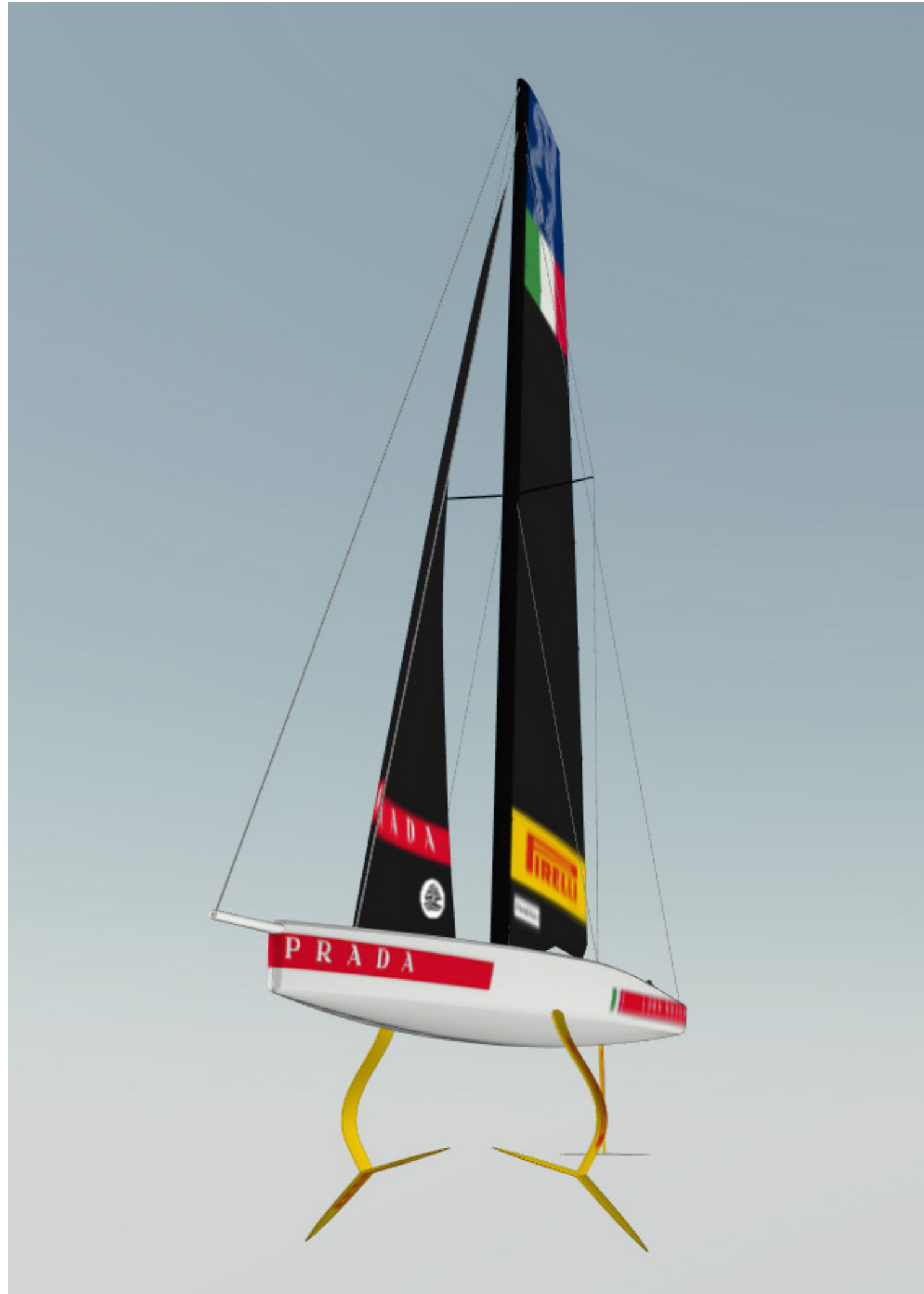
Dock configuration: both foils lowered, minimum beam
